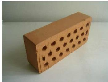
Figura 18.2 Esempio di mattone semipieno  $15\% < \phi \leq 45\%$  in laterizio per murature portanti (fonte: [www.fornacetrezzo.it](http://www.fornacetrezzo.it))
